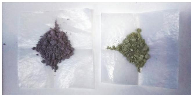
図4 CuAlO<sub>2</sub>とCuGaO<sub>2</sub>の粉末
